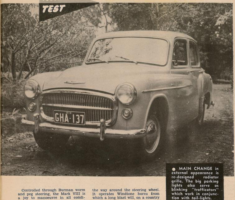
Controlled through Burman worm and peg steering, the Mark VIII is a joy to manoeuvre in all conditions. Requiring only two turns of the helm to take the front wheels from one lock to the other, the whole car can be turned in 33ft.
